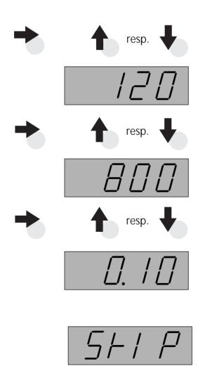
Example: The biscuit firing 800°C (refer to table shown above) is entered as a firing curve as follows:
