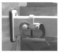
The connection is secured with the retaining clip.
