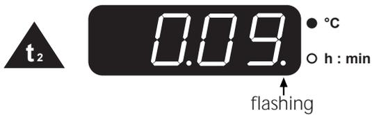
Note that when checking  $t_1$  or  $t_2$  only the remaining time of the segment is shown.
