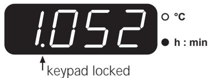
To prevent the PYROTEC D1 from unauthorized usage you can lock the keypad by pressing the key (4). A decimal point on the left hand side in display (1) indicates the controllers keypad is locked. If the controller is locked you can check values but not for instance start or interrupt a firing.
